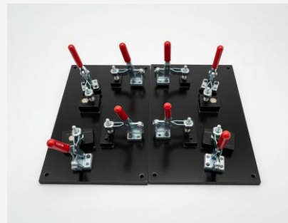
Custom Fixture Plate – Multi-part clamping
