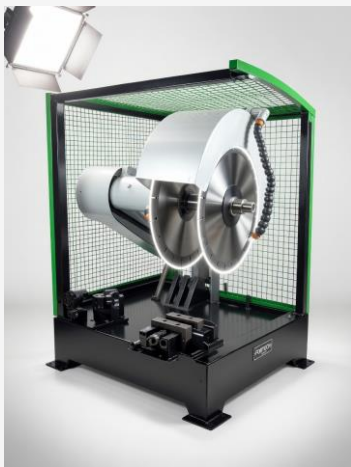
SPM Casting Cutting – Auto feed, guarded (Customer: Mahindra)
